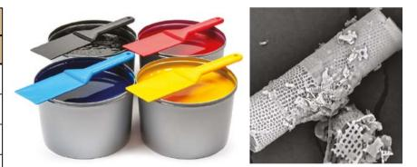
The diatoms in Celatom fine fillers contain about 85% void space, which increases the permeability of the paint film. Increased permeability allows the paint vehicle to rapidly volatilize so the paint dries quickly and uniformly. This produces a more durable coating with reduced blistering and peeling. Besides providing sheen control, Celatom fillers also increase coating durability and toughness.
